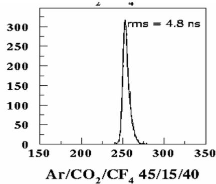
The results of several tests\* on 10x10 cm<sup>2</sup> prototype allowed us to select the **Ar/CO<sub>2</sub>/CF<sub>4</sub>** with geometry **3/1/2/1 mm**
