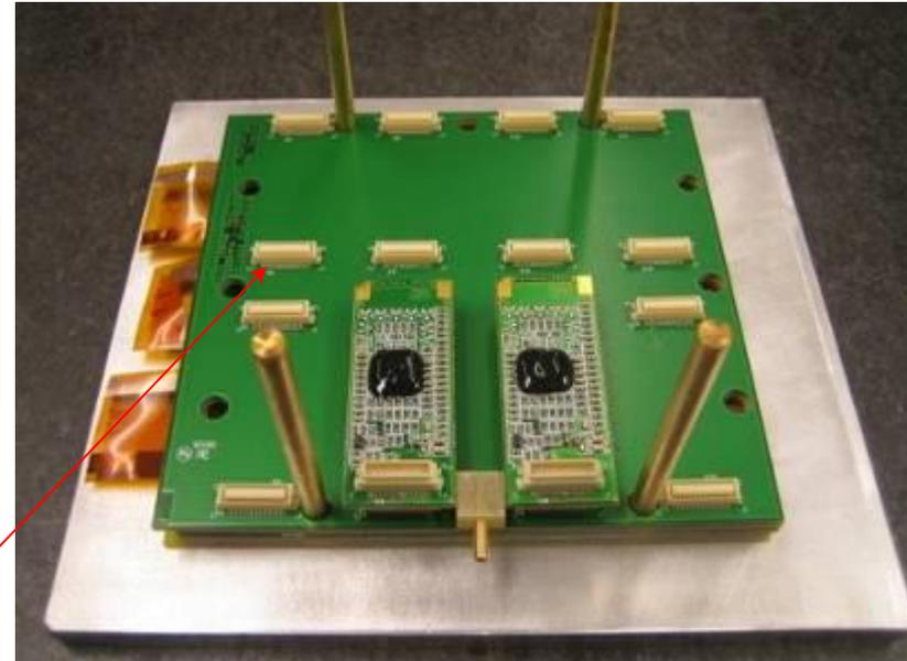
All the anode PCB have been designed with the **same connector layout** for a total of **128 channels** (1ch/cm<sup>2</sup>)
