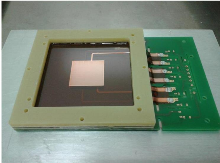
The detector could be open again and the ceramic board with 4 medipixes could be changed at any time
