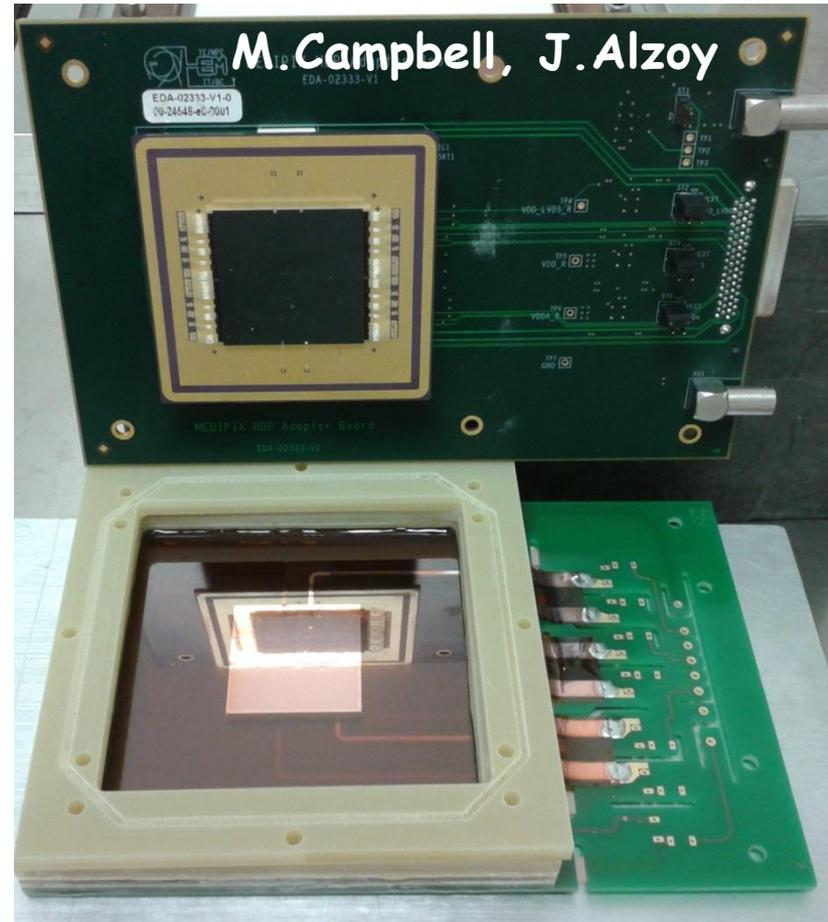
The chamber gain has been increased to produce small sparks on GEM foils: no effect on medipix chip
