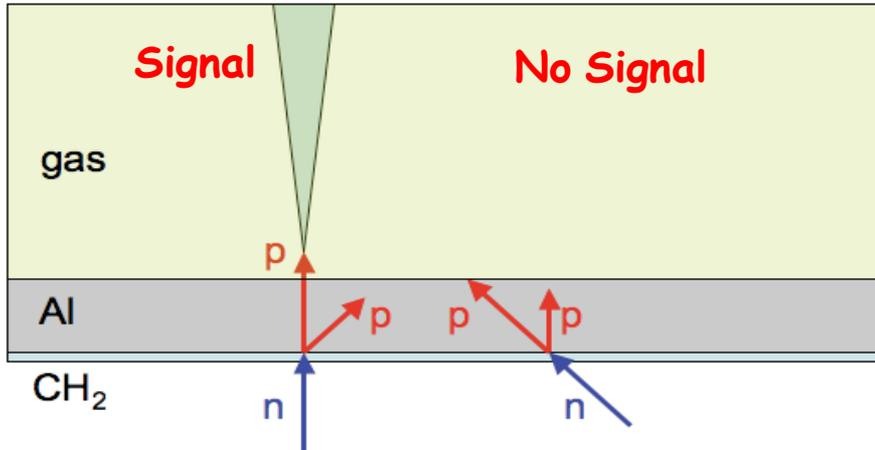
Optimized  $\text{CH}_2$ -Al thicknesses ( $50 \mu\text{m}$ - $50 \mu\text{m}$ ) determined by simulations (MCNPX-GEANT4)
