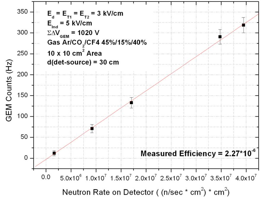
Good linearity measured up to 4x10<sup>7</sup> neutron/sec cm<sup>2</sup> the maximum rate reached by this facility
