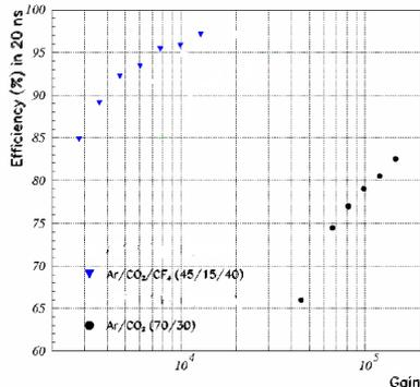
→ higher efficiency at **lower gas gain : 96% in 20 ns**
