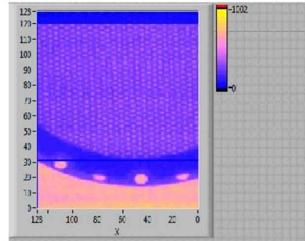
These images was realized in real time moving a triple gem with an array of 128 pads 0.5x0.5 mm crossing the beam
