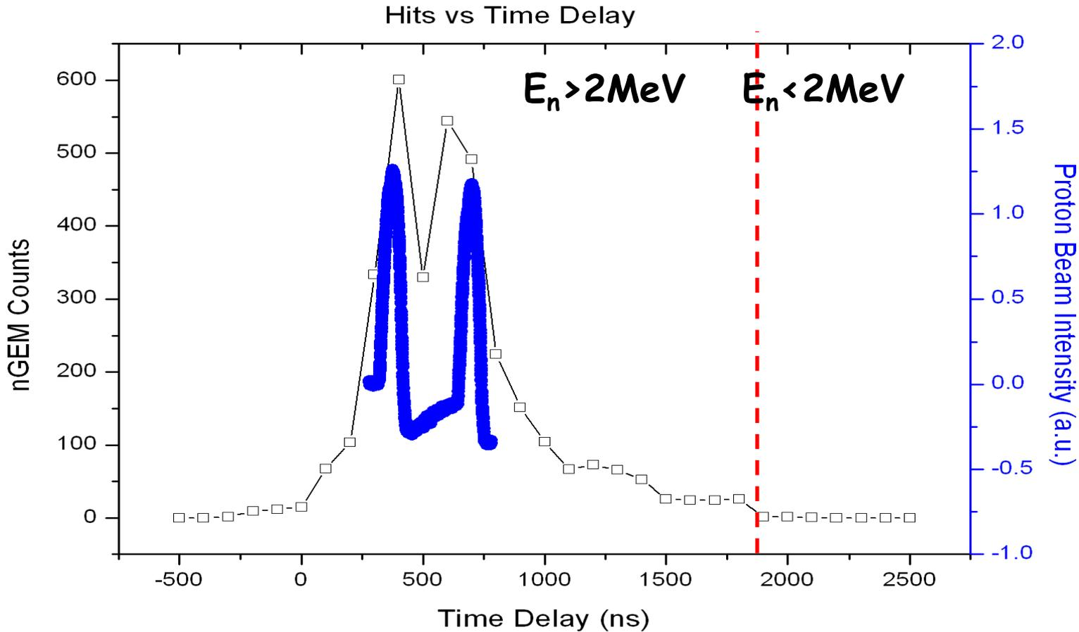
Rate measurement scan on time delay from beam  $T_0$  using GEM detector with **100 ns gate**.
