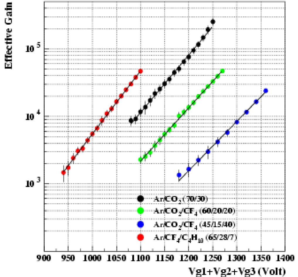
$$G_{\text{eff}} = A e^{\alpha(V_{\text{gem1}}+V_{\text{gem2}}+V_{\text{gem3}})}$$
