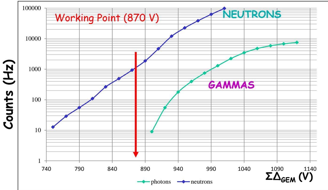
Counting rate Vs chamber gain: up to 890 V the chamber is sensitive to fast neutron but not to gamma rays.
