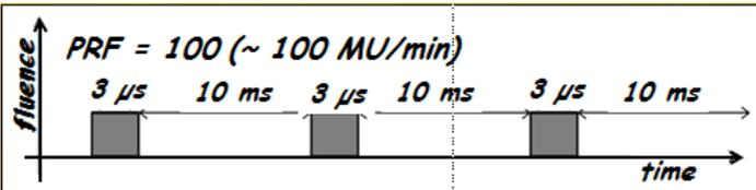
*Scheme of the beam flux pulsed time structure of the Elekta Synergy Linac at PRF = 100 MU/min.*
