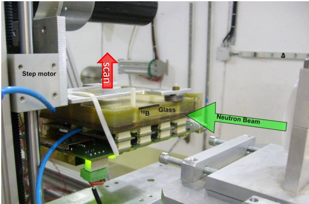
With a scan procedure it is possible to make an image of the neutron beam in the thermal region
