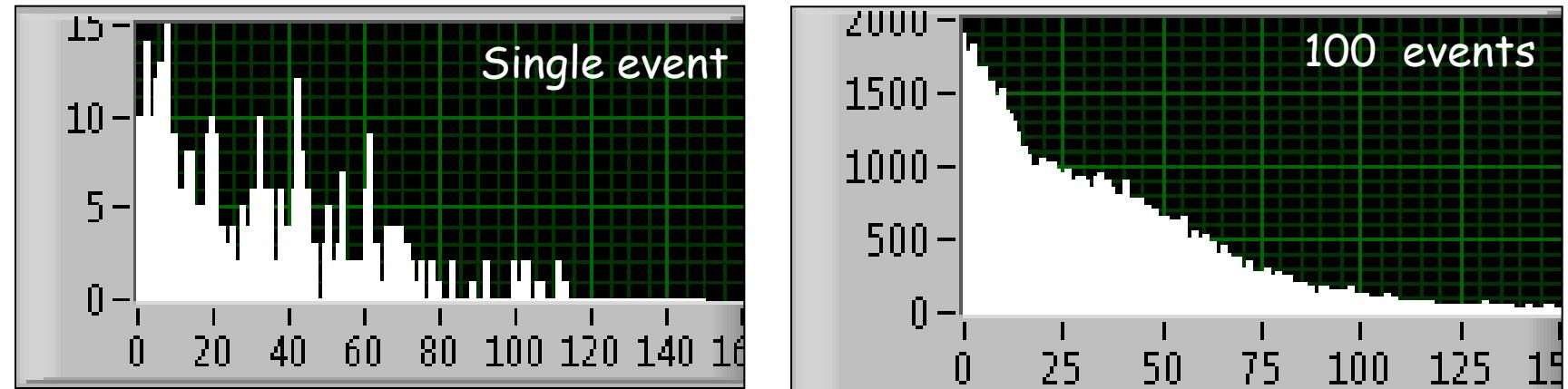
Slices acquisition: Time spectrum (1ms/bin), 150ms total gate.
