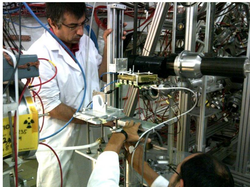
Neutrons are collimated and guided through an evacuated beam pipe to an experimental area at **185 m** from the spallation target.
