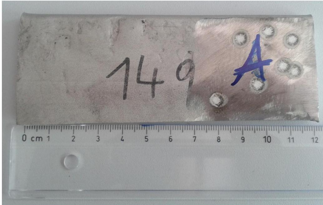
Sample from STS pipes with well known isotope composition from radiochemical analysis and gamma spectroscopy.
