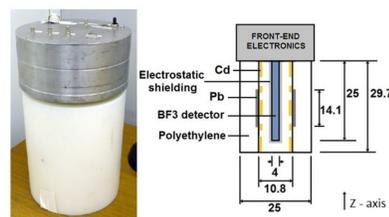
Figure 2. The LUPIN-II detector (all dimensions in cm)
