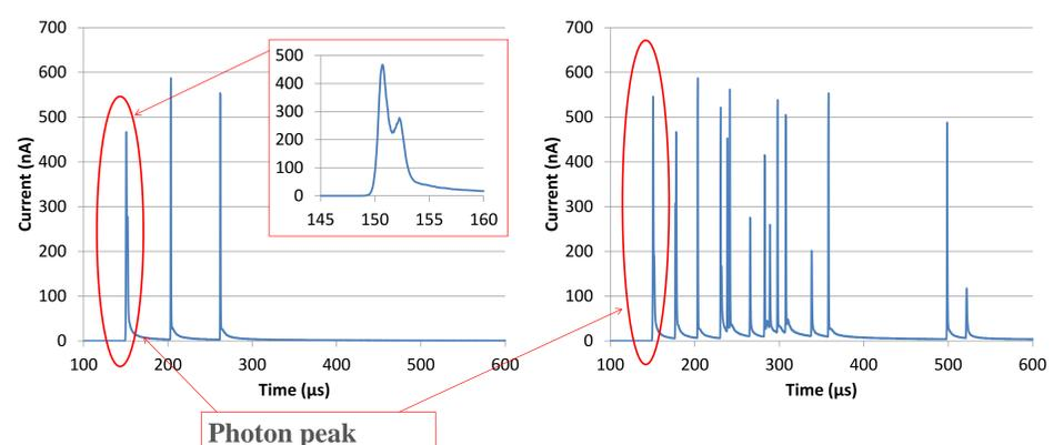
For these results, the photon peak corresponded to a value of 3 neutrons. Thus, for this field, the detector output was modified by 3 neutrons/burst to compensate.
