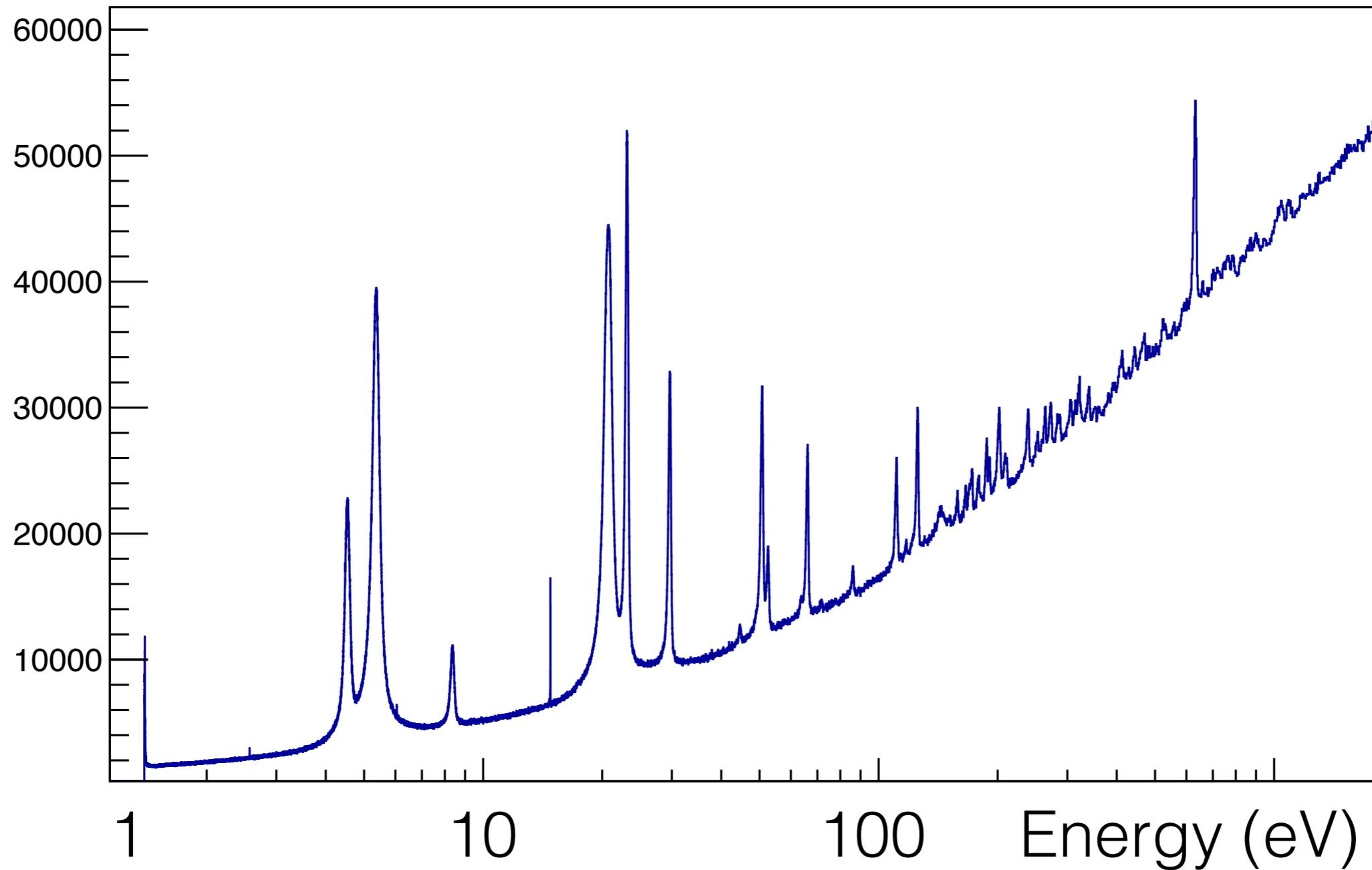
Neutron/gamma interactions with gold in the PCB board, lead in the solder bumps and gadolinium in the collimator
