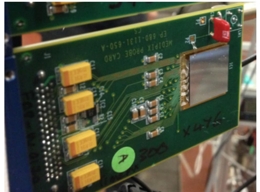
**Timepix mounted on CERN probe card**
