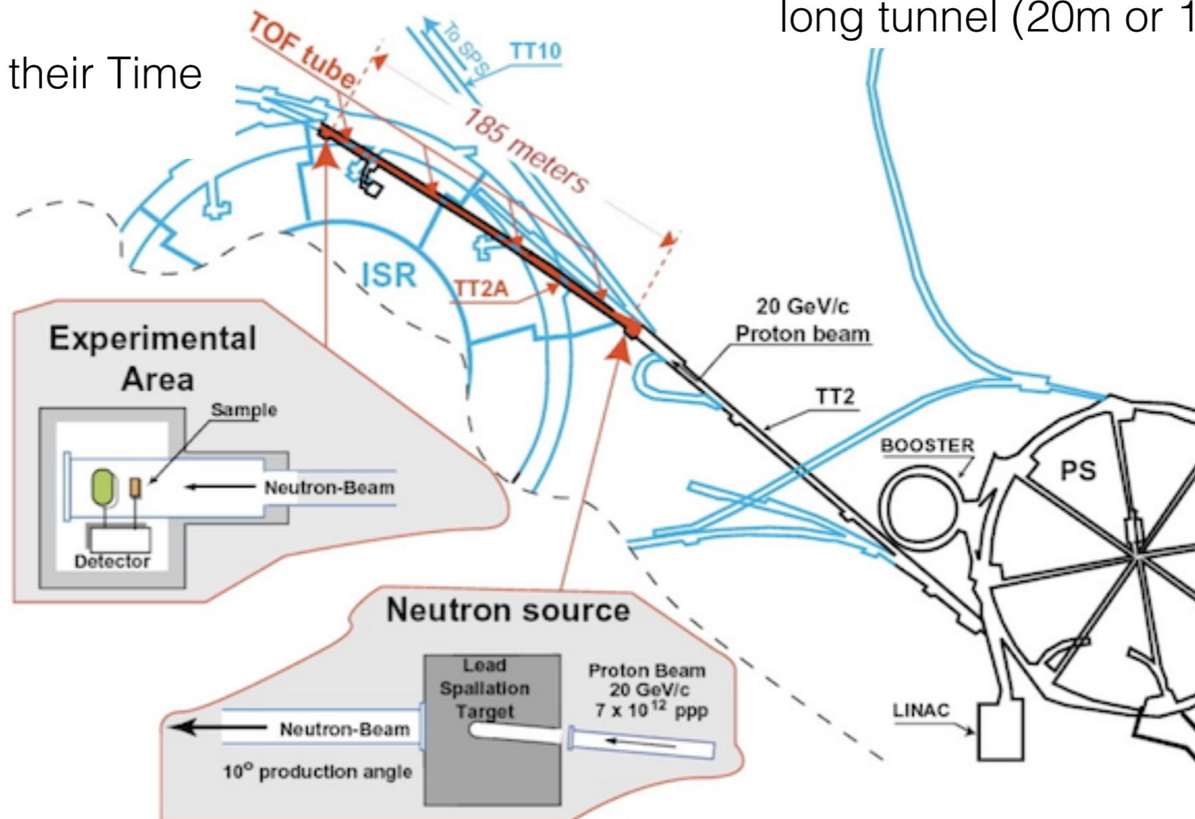
(1) PS Protons collide with a lead target producing neutrons
