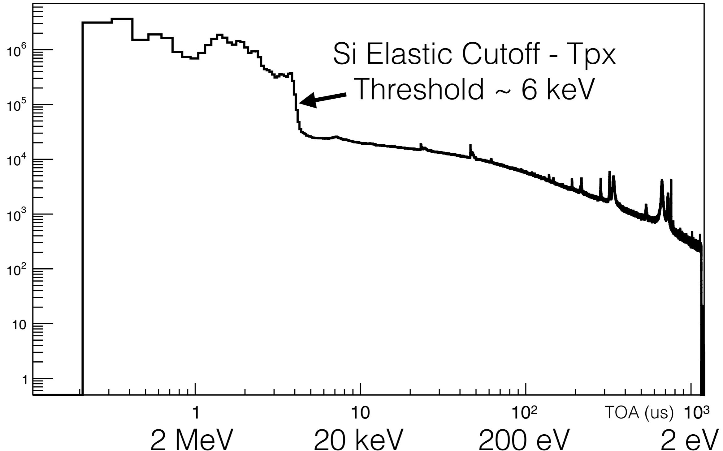
~3000 spills (~ 5 hrs), timepix with boron + plastic converter
