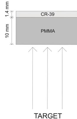
Fig 2. Layout of the passive detection system at the position CT 12 which is right on top of the irradiated target (neutron source).
