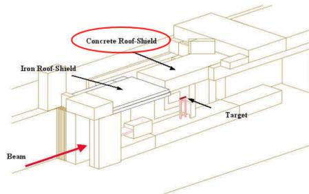
Fig 1. Complex neutron field on the concrete Roof-Shield situated right above the irradiated target
