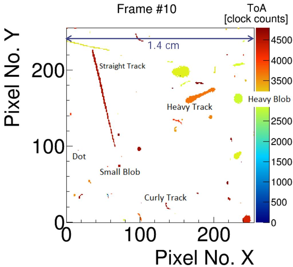
Frame taken with a Timepix (1 mm, 400V,  $t_{\text{Acq.}} = 100\mu\text{s}$ ) in the LANSCe neutron beam.
