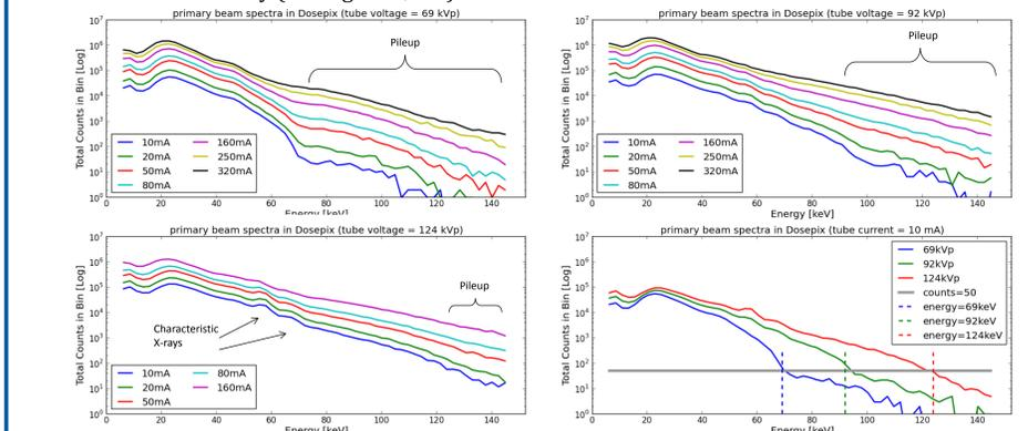
Figure 6. Dosepix measurements of the primary beam spectra, with the beams programmed with: 69 kVp and varying tube current (top left), 92 kVp and varying tube current (top right), and 124 kVp and varying tube current (bottom left), and 10 mA tube current and varying tube voltage (bottom right). The data shown here has not been processed; energy binning was done on-chip.
