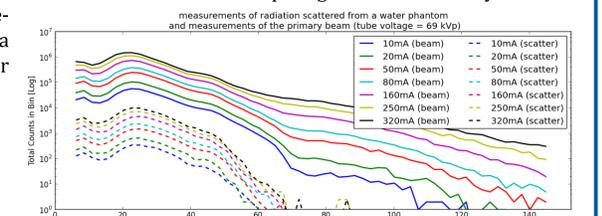
Figure 10. Dosepix measurements of radiation scattered from a water phantom. Measurements from the primary beam are included for comparison.
