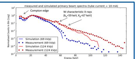
Figure 8. Simulated spectra of the primary beam absorbed by the detector materials. Spectra measured by Dosepix are included for comparison.
