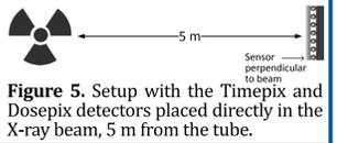
Figure 5. Setup with the Timepix and Dosepix detectors placed directly in the X-ray beam, 5 m from the tube.
