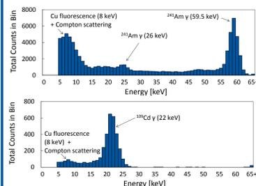
Figure 4. Spectra measured by Dosepix exposed to <sup>241</sup>Am (top) and <sup>109</sup>Cd (bottom)
