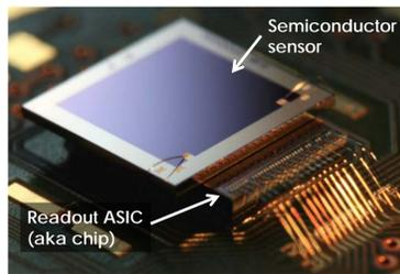
Figure 1. Photograph of the Dosepix hybrid pixel detector (courtesy of ECAP, Erlangen)
