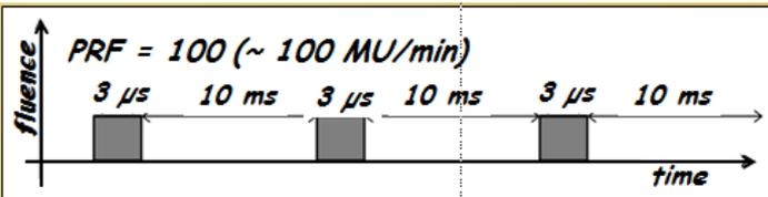
Scheme of the beam flux pulsed time structure of the Elekta Synergy Linac at PRF = 100 MU/min.
