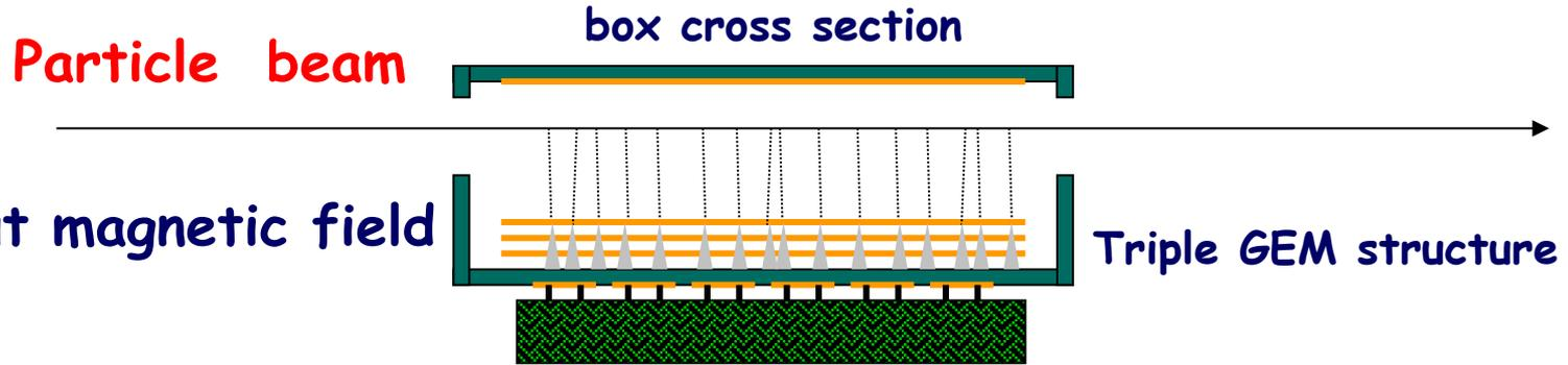
The material budget crossed by a particle is only two kapton foils ( $<0.2\%X_0$ ) used for the field cage necessary for the drift field uniformity
