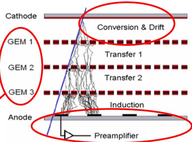
Working with different levels of gain it is possible to obtain **high level of particle discrimination**
