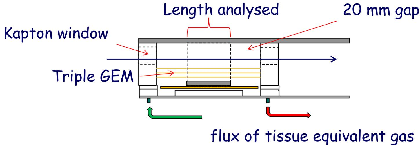
The particle track is analysed with 512 pixel in 3 cm length
