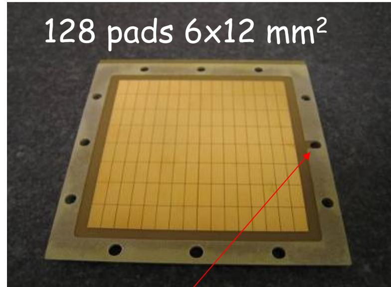
The frame for the G3 foil has been modified for the gas inlet
