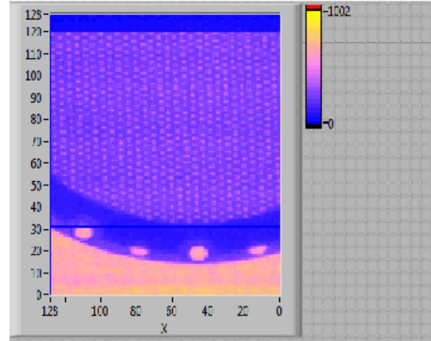
These images was realized in real time moving a triple gem with an array of 128 pads  $0.5 \times 0.5 \text{ mm}^2$  crossing the beam
