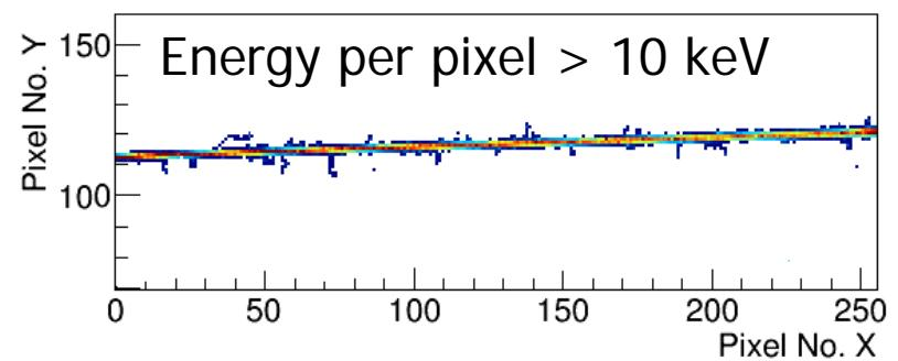
**Identify particle type and particle energy via the size of the halo, the number of delta rays, their length and  $dE/dx$ .**
