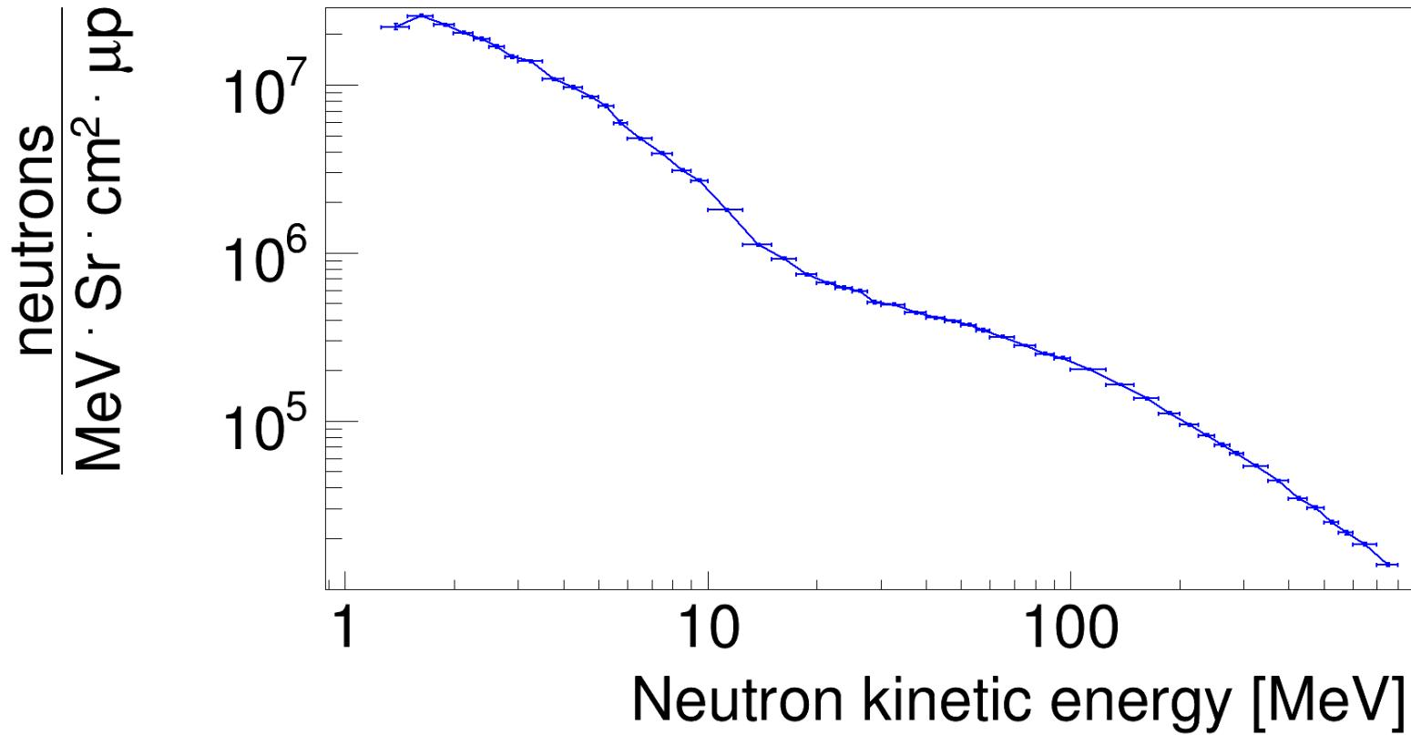
Energy spectrum of the neutrons measured by a  $^{238}\text{U}$  fission chamber
