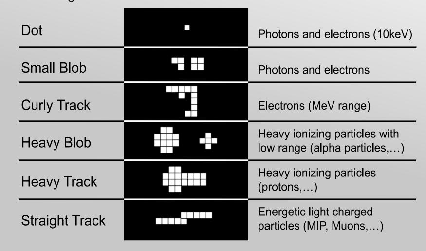
Particles that locally deposit a huge amount of energy in the Silicon sensor layer are further referred to as "High Energy Transfer Particles" (HETP). Their signatures are Heavy Tracks and Heavy Blobs. In terms of neutron detection, this HETP-signatures are created by the recoiled protons below PE and nuclear interactions of neutrons in the Silicon itself.
