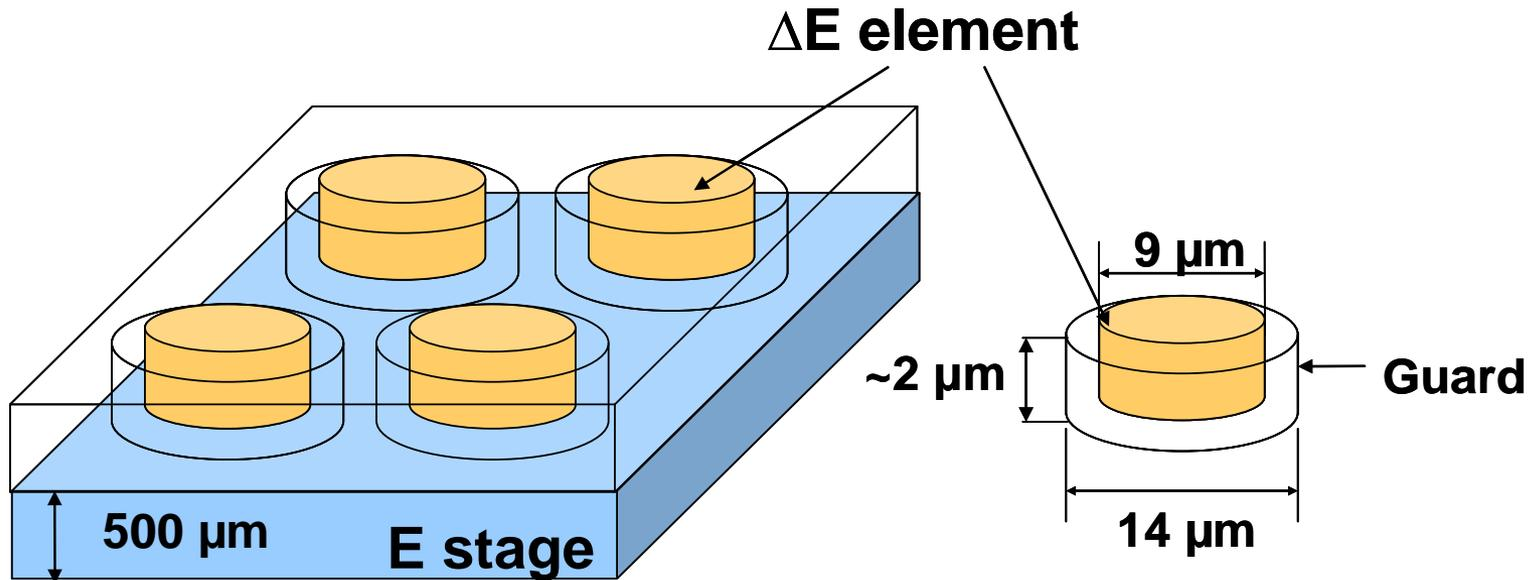
More than 7000 pixels are connected in parallel to give an effective detection area of the  $\Delta E$  stage of about  $0.5 \text{ mm}^2$
