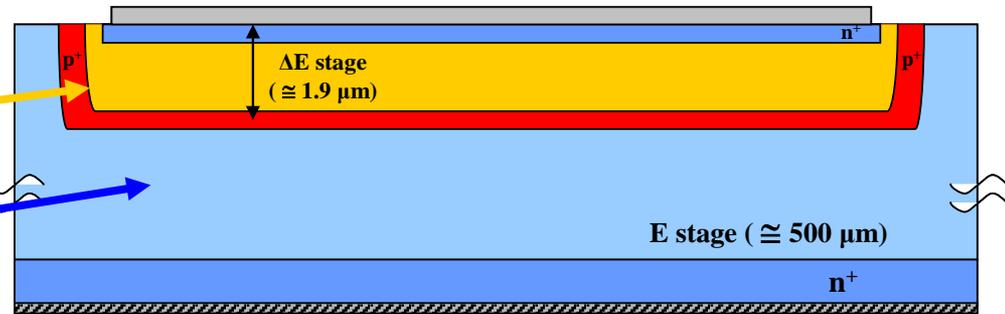
**$\Delta E$  stage** : matrix of cylindrical diodes ( $h = 2 \mu\text{m}$  ,  $d = 9 \mu\text{m}$ )
