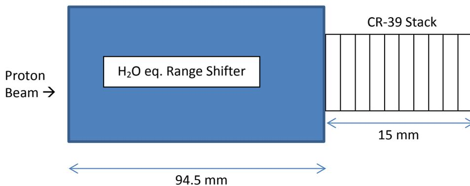
Figure 2. Experimental setup with Proton beam
