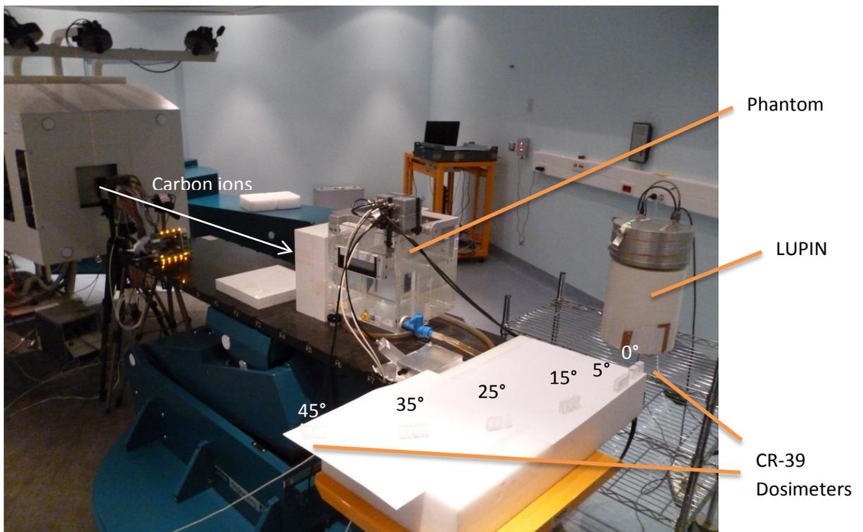
Figure 7. Illustration of the detectors' dispositions around the phantom
