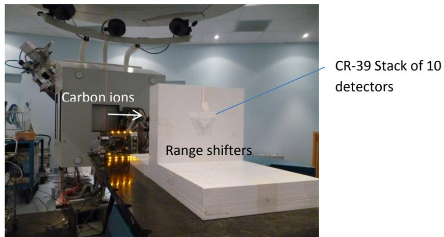
Figure 4. Experiment 2 and 3 have the same configuration as in Experiment 1 but the beam is changed to the Carbon ions.
