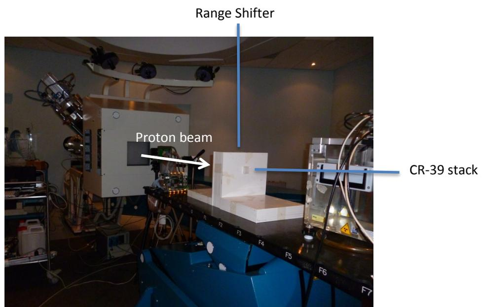
Figure 1. This picture shows the experimental setup with the beam direction represented by the white arrow incident on the range shifter acting as a water equivalent phantom and the CR-39 stack placed behind the range shifter.
