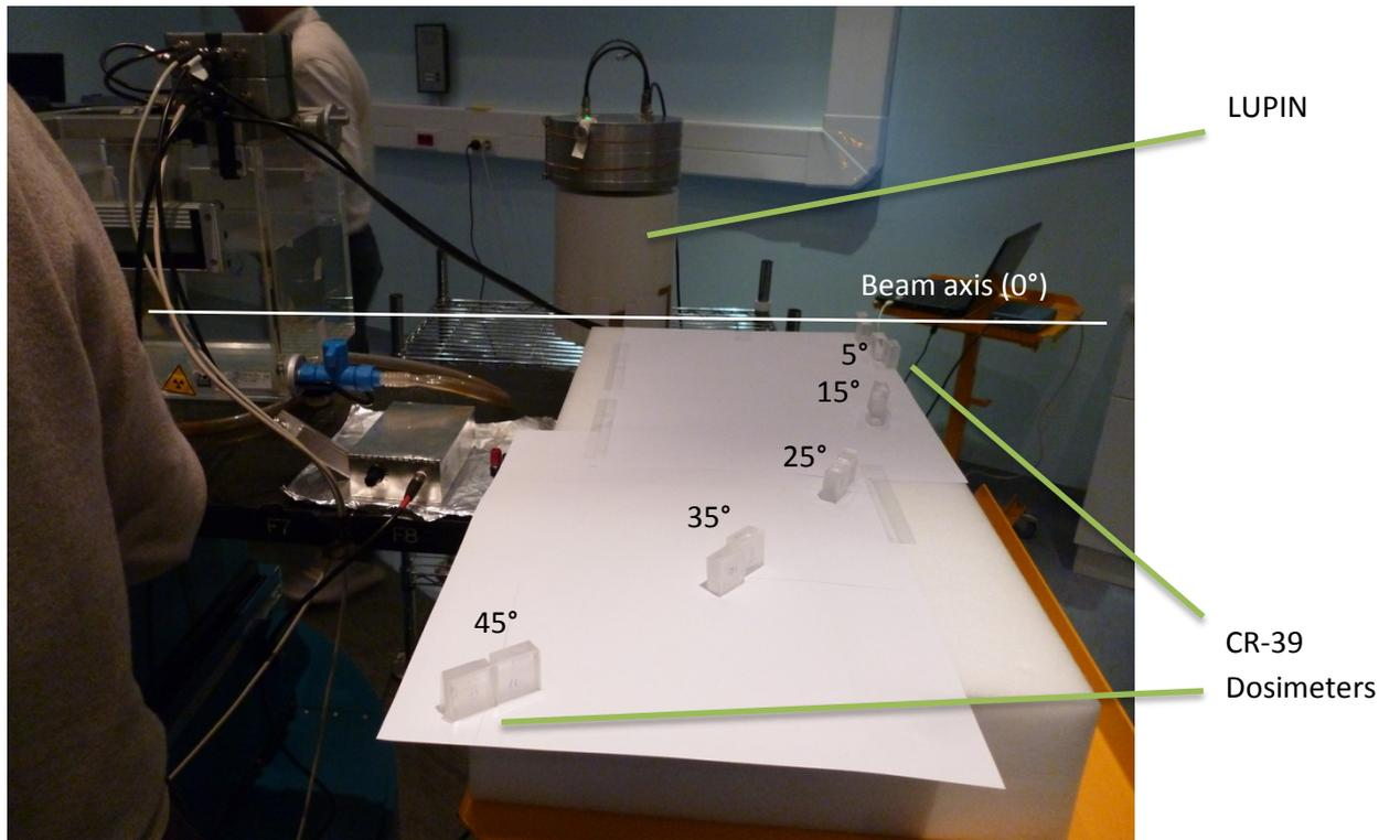
Figure 8. Positioning of the LUPIN and the CR-39 based dosimeters around the beam axis.
