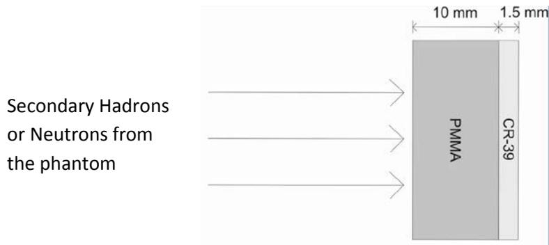
Figure 6. Illustration of the CR-39 based dosimeter
