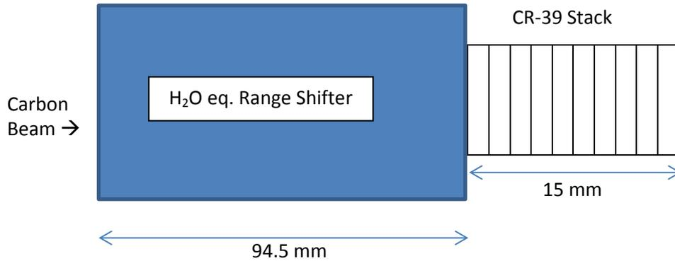
Figure 3. Experimental setup with Carbon ions beam
