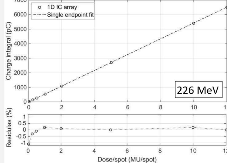
Detector response for different energies is linear within ±1%. Measured dose ranges from 5cGy up to 30Gy.
